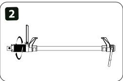
2. Fully loosen nut by turning counterclockwise.
